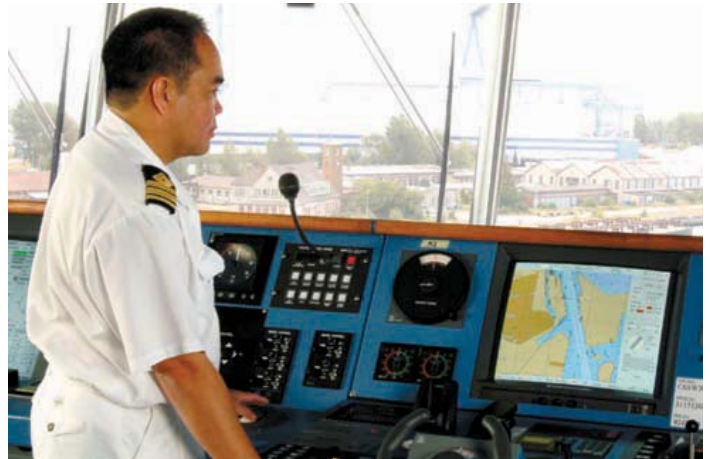
Electronic charts and ECDIS can make it easier to update folios, and may also reduce the burden on the navigator
